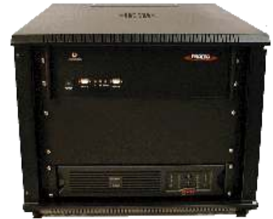
Rack Mounted with UPS
